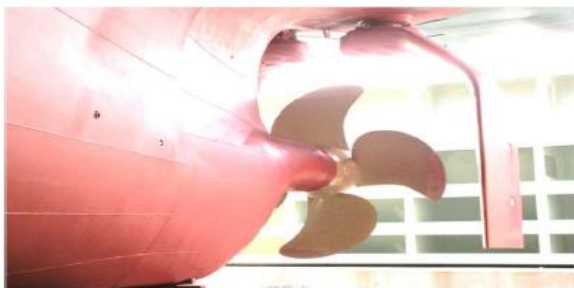
The Gate Rudder installed on Shigenobu
