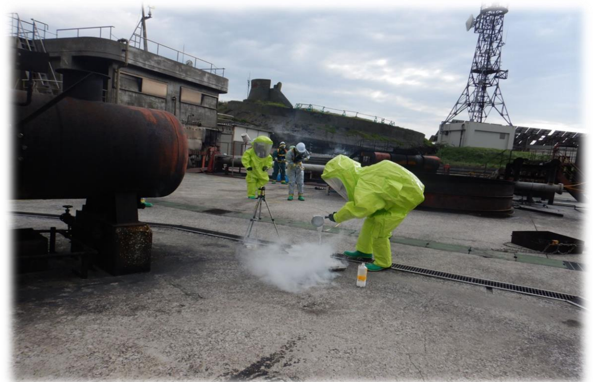
Dispersion experiment of ammonia
