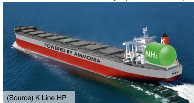
Ammonia fueled ship (bulk carrier)
